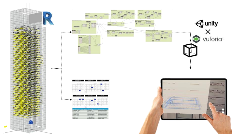
Figure 4. BIM–Digital Twin–XR architecture overview of the TRP pilot for electrical maintenance, showing the Revit-based model environment, identifier-based data structuring, maintenance data extraction, and AR visualization through Unity and Vuforia.
