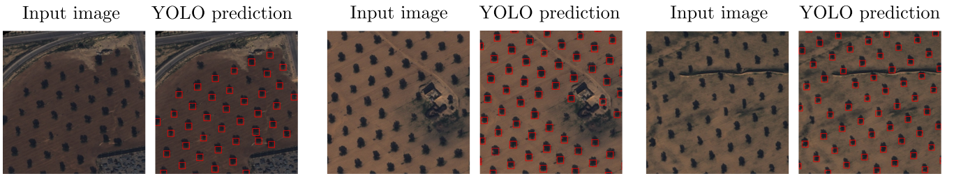
Fig. 7. Examples of detections produced by the YOLO-V8-l model on real RGB+NIR satellite imagery. The input tiles are displayed as RGB composites extracted from the four-channel data, and the red bounding boxes indicate the predicted locations of individual trees. The count of detections in each image was used as the estimated tree count.
