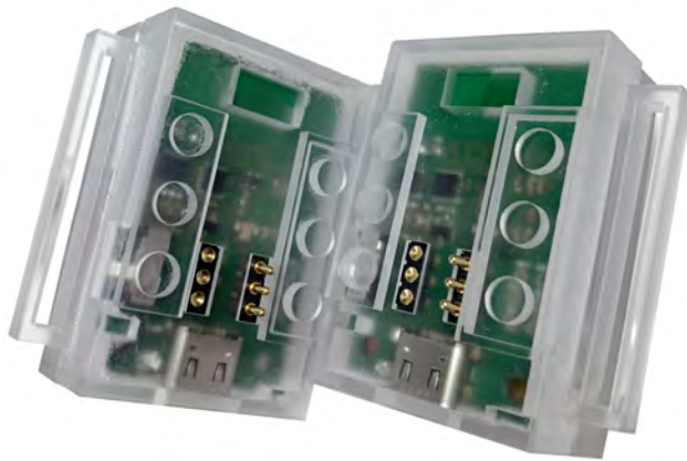
(a) Wearable enclosures (45x42x20)mm
