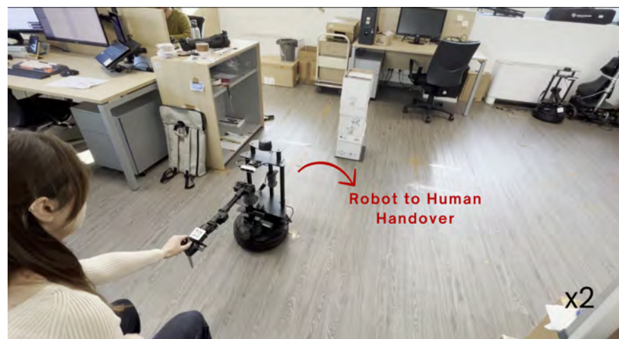
Figure 15. Robot-to-human item handover process.
