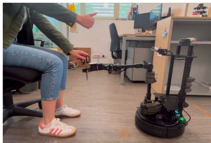
Figure 16. The user shows the thumbs-up gesture to communicate the success of the delivery to the robot.
