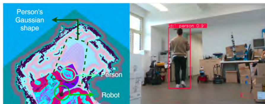
Figure 14. Safe navigation behavior of the mobile manipulator. (Left) RViz visualization of the person's Gaussian shape. (Right) Robot's point of view of the identified person.
