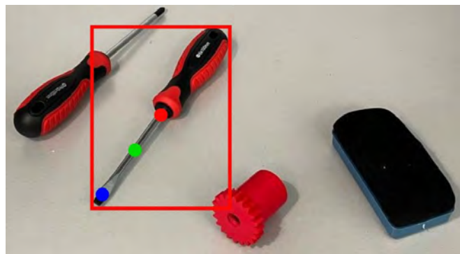
Figure 2. Predicted grasping point (red), point indicated by the user (blue), and grasping point for the robot (green).
