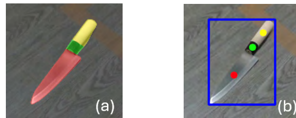
Figure 4. (a) Affordance mask and (b) affordance keypoints of a knife. Red, green, and yellow marks refer to danger , grasp , and handle affordances, respectively.
