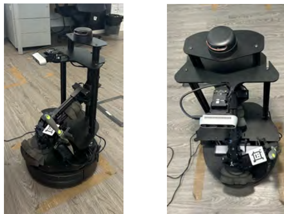
Figure 10. Safe position of the manipulator after picking up the requested item. Lateral view ( left ) and top view ( right ).
