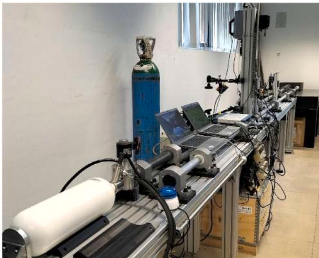
Fig. 3. DIHPB experimental setup for high strain rate tests.
