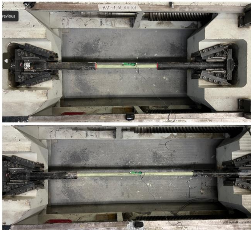
Figure 15. Test setup for each FRP bar at both gauge lengths
