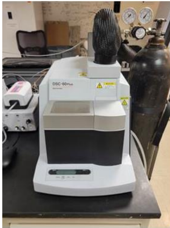
Figure 29. Test setup showing DSC in operation
