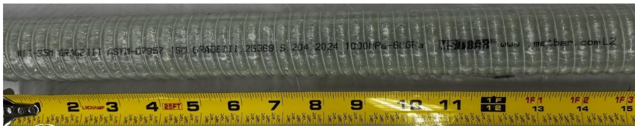
Figure 26. FRP straight bar #11 manufactured by MST-Bar.
