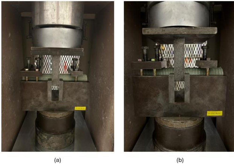
Figure 34. Transverse shear strength test setup (a) Pultrall and (b) MST-Bar
