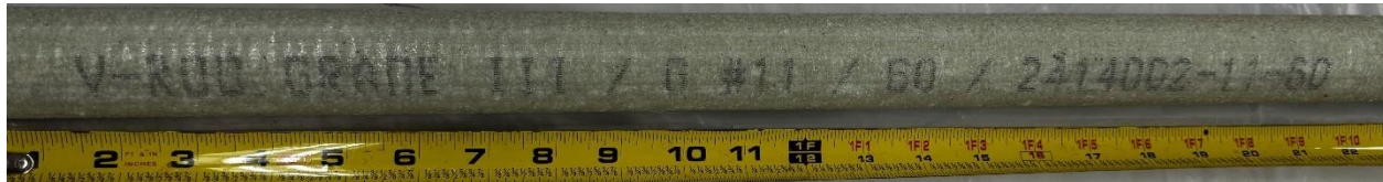
Figure 25. FRP straight bar #11 manufactured by Pultrall.
