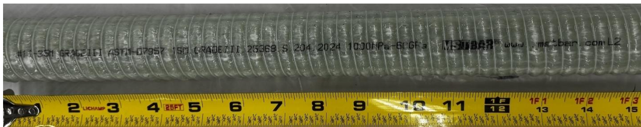
Figure 26. FRP straight bar #11 manufactured by MST-Bar.
