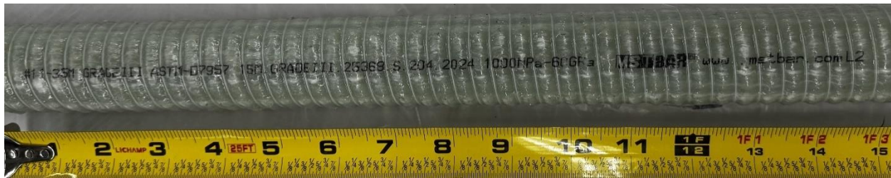
Figure 26. FRP straight bar #11 manufactured by MST-Bar.
