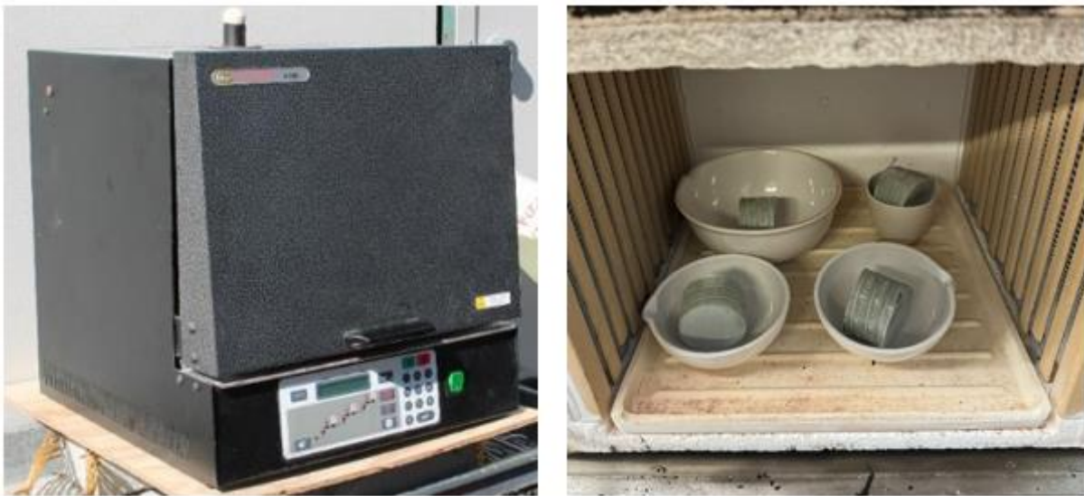
Figure 27. Fiber content furnace test setup
