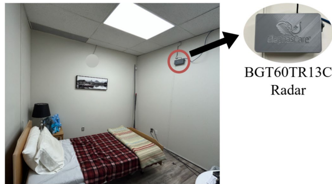
Fig. 3. Room layout and radar placement in the home-like data collection environment.
