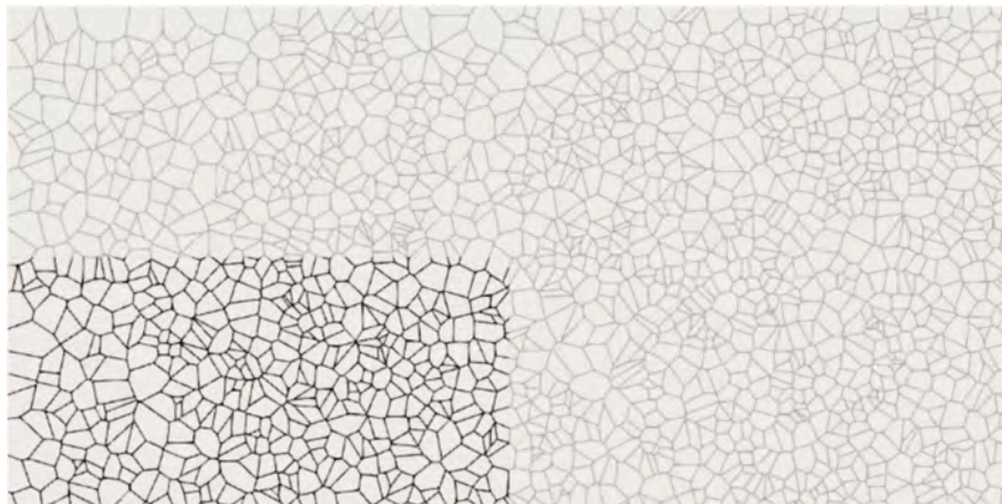
Fig. 6. Voronoi subset (black) used as porous domain in two-phase flow simulation. The porous area simulated in the monophase scenario shown in light grey.
