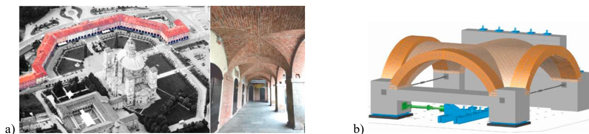
Fig. 1. (a) the “Palazzata” cross-vaults of the Sanctuary Regina Montis Regalis of Vicoforte, Italy (from Alforno et al. 2024); (b) testing rig for the seismic assessment of twin masonry cross-vault specimens from the cloister.
