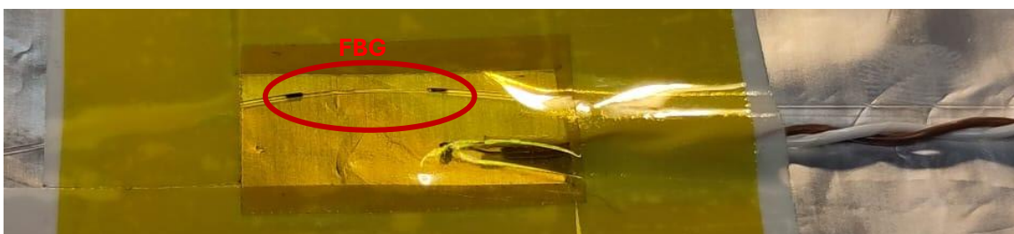
Figure 5. FBG and thermocouple detail during thermal calibration process
