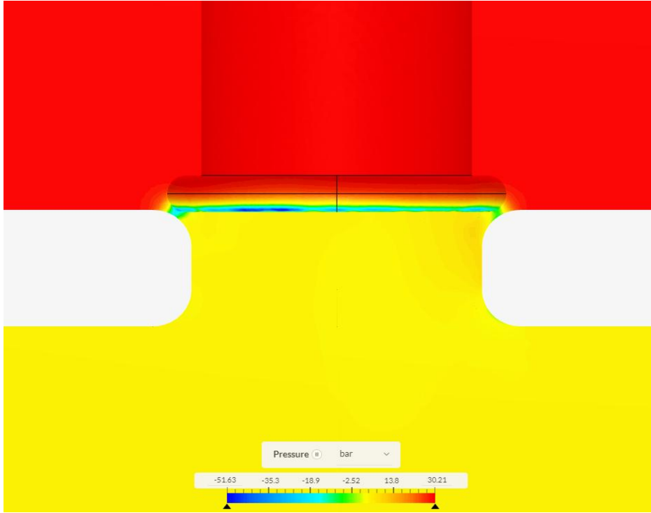
Figure 15 Pressure field of the LH2 flow around the non-optimized piston body.
