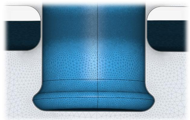
Figure 7 Volume Mesh with Tetrahedral cells.
