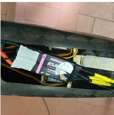
Figure 7 – FBG on the ESC (left) and on the battery (right)
