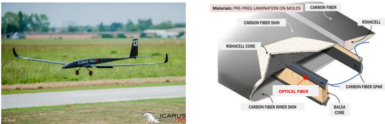
Figure 1 – The Anubi UAV (left) and a detail of the wing's structure with optical fiber (right)
