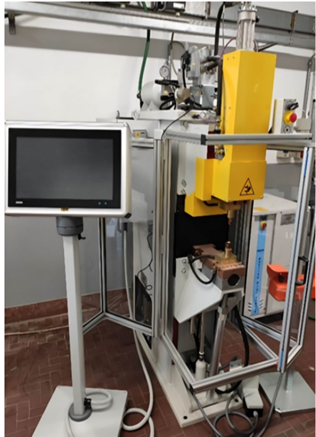
Fig. 2 RSW machine used during the experimental campaigns
