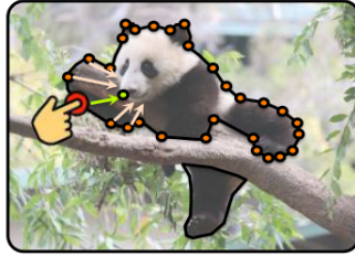
Figure 8: Example of polygon interaction: the user can select any incorrect control point and move it to the boundary to correct the output mask. Image from [102].
