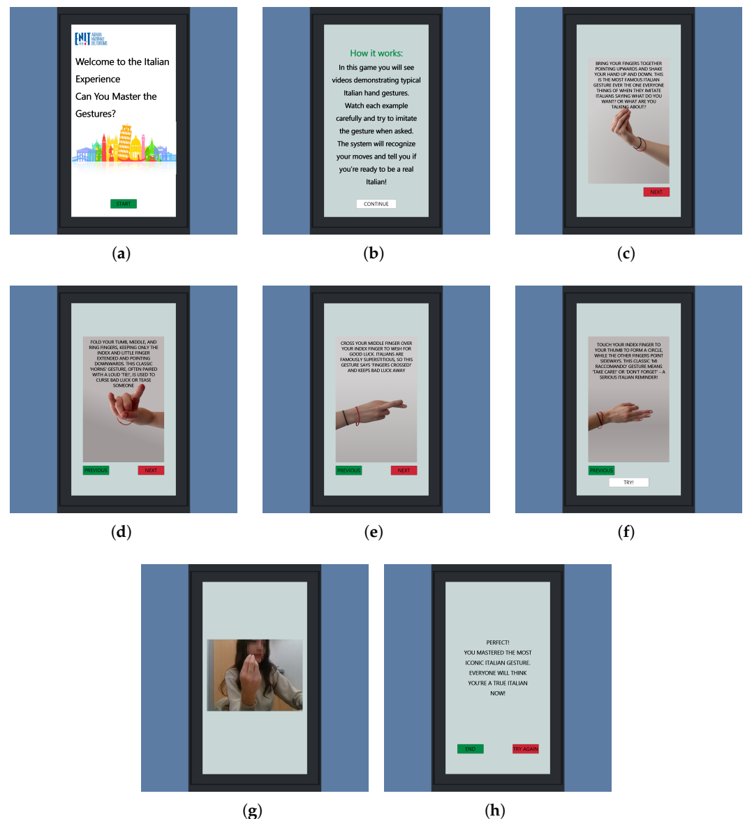
Figure 5. Screenshots of the developed Unity-based application simulating an interactive airport information totem for learning Italian hand gestures. The figure illustrates the complete interaction workflow, from instructional content presentation to user gesture performance and real-time automatic recognition with visual feedback. (a) Home interface of the virtual totem. (b) Tutorial interface for gesture learning. (c) Single gesture instructional view. (d) Horns instructional view. (e) Crossed fingers instructional view. (f) Perfection instructional view. (g) User performing a gesture in front of the totem. (h) Real-time gesture recognition and feedback display.
