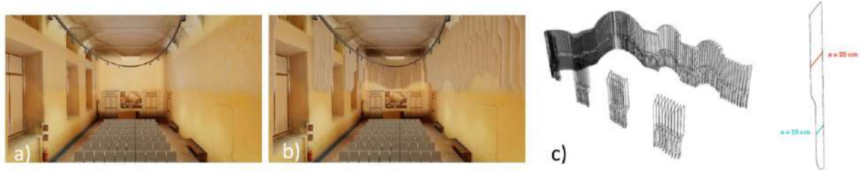
Figure 4: Rendered images of the two solution strategies: a) with multilayer fibrous sound absorbing panels and b) parametrically designed acoustic baffles. c) Parametric baffles structure.
