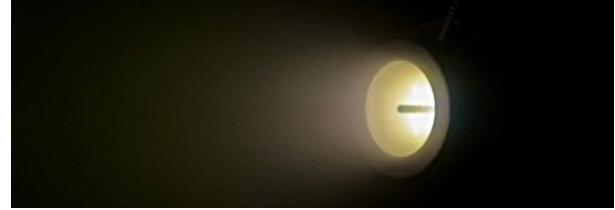
Fig. 3. Photo of ECRA thruster operated with iodine inside ONERA facility, at a volume flowrate of 1.5 sccm, 25 W of input power, at a pressure of 1.65 \cdot 10^{-5} mbar (without cryogenic system).
