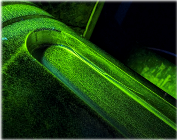
Figure 7. Crack nucleation present in a tested shaft.
