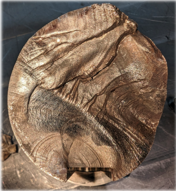
Figure 2. Shaft failure section.
