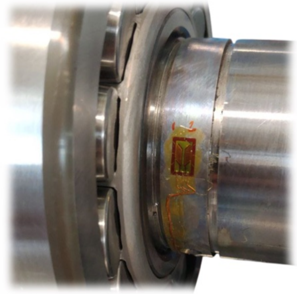
Figure 4. Part of full bridge strain gages used to measure torque transmitted by the shaft.
