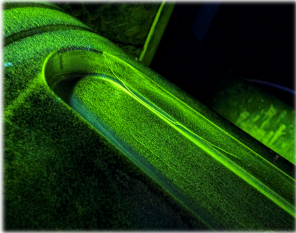
Figure 7. Crack nucleation present in a tested shaft.
