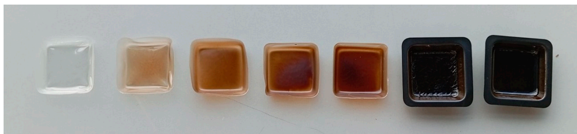
Figure 4. The visual appearance of PVA/BSF protein films in % w/w 100/0, 90/10, 70/30, 50/50, 30/70, 10/90 and 0/100 from left to right.
