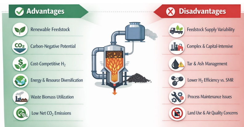
Figure 5. Summary of advantages and disadvantages of biomass gasification.
