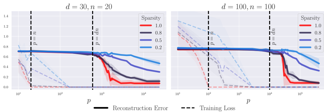
Figure 16: Thresholds for label fitting and data reconstruction of pruned models. We consider RF regression with ReLU activation, fitting a noisy linear model. The training data is i.i.d. uniformly drawn from the d -dimensional sphere. After fitting, we prune the trained parameters \theta^* with Optimal Brain Surgeon (Hassibi & Stork, 1992) to a desired sparsity ratio ( i.e. , p'/p with p' the number of remaining parameters). We report mean (solid/dashed lines) and standard deviation (shaded areas) for both the reconstruction error (solid lines) and training loss (dashed lines) as the number of parameter p increases, at different choices of input dimensions d and number of samples n . Statistics are computed across 10 distinct random seeds. Lighter colors refer to lower sparsity ratios, compared against the unpruned baselines (red lines).
