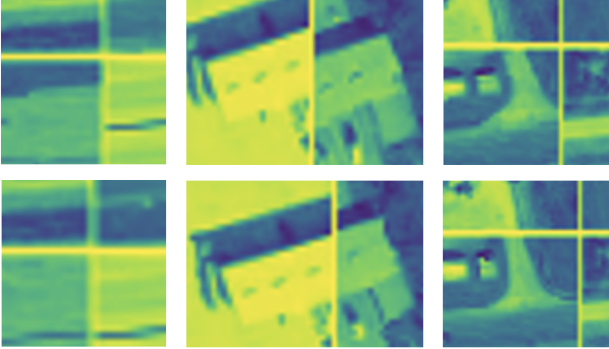
Fig. 2. Qualitative comparison of image registration using a chessboard made of alternated patches from a source image and the warped (registered) image. Top Row: registration performed by Solo-Reg pretrain; Bottom Row: registration performed by Reg-CD pretrain.
