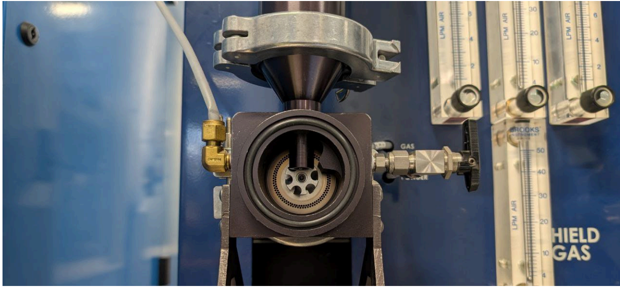
Fig. 1: Optomec CS 150 powder feeder system metering chamber.
