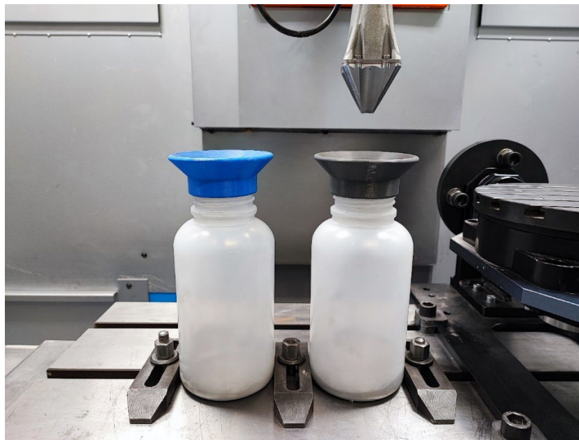
Fig. 3: Experiment setup for powder mass flow rate.
