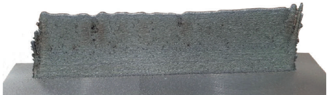
Figure 5. Surface re-melting in the DED process, illustrating the waviness error on the deposited surfaces with overall dimensions (120 \times 50 \times 20) \text{ mm}^3 [37].
