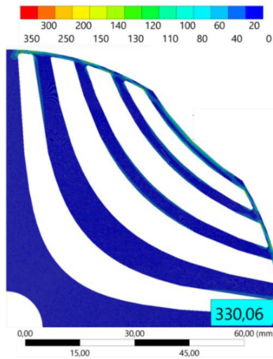
FIGURE 4. Equivalent Von-Mises stress at the maximum speed (8000 r/min).
