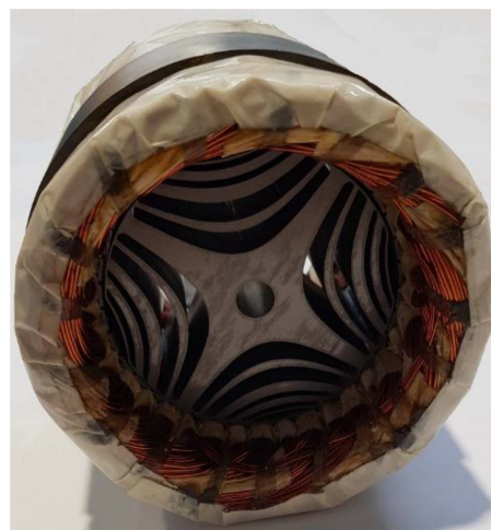
FIGURE 5. Manufactured SynRel prototype.
