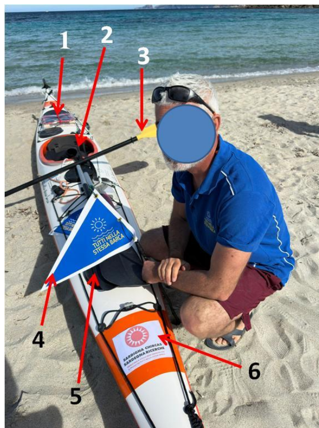
Figure 1 The kayak and its kayaker. (1) photovoltaic panel; (2) cockpit; (3) paddle; (4) pennant bearing the expedition name; (5) watertight bow locker containing scientific instruments; (6) adhesive panel bearing the logo of Sardegna Ricerche, the Italian research institution that provided patronage for the experiments together with the Polytechnic University of Turin in Italy.
