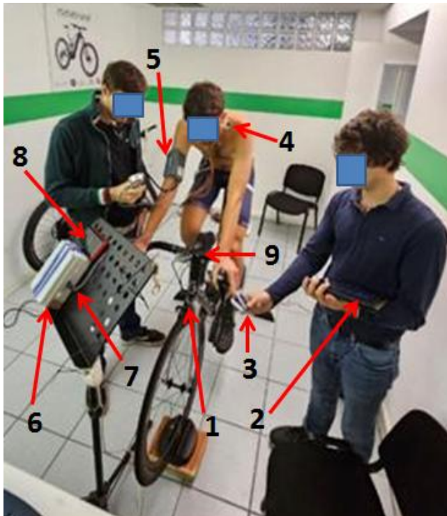
Figure 4 Image of a tested cyclist, assisted by two skilled operators from the Polytechnic University of Turin, Italy, while pedaling on his bike. (1) The rear wheel has been replaced with an Elite Direto XR-T power meter (not visible in the image). (2) Tablet organizer held by one of the operators for acquiring mechanical and biomedical measurements, the latter manually recorded by both operators. (3) Finger pulse oximeter. (4) Disposable ECG electrode visible here, attached at the roots of the neck muscles. (5) Inflatable sphygmomanometer cuff with stethoscope, used by the other operator to auscultate brachial artery sounds. (6) Box containing the E-Physio impedance cardiograph hardware and electronics. (7) Five-pin connection cable linking the athlete's chest electrodes to the impedance cardiograph. (8) Power bank providing 5 V, 2.4 A DC supply to the impedance cardiograph. (9) Garmin Edge cycle computer.
