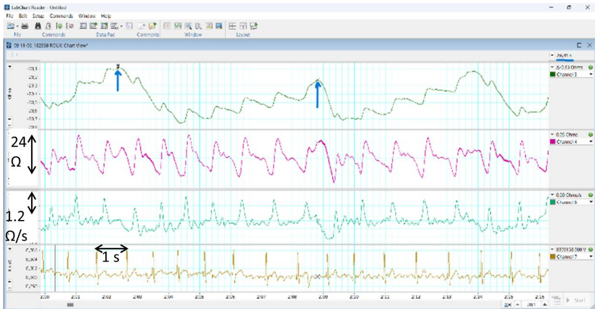
Figure 3 Analog traces of bioimpedance variables recorded by the LabCart Reader from a cyclist at rest. From top to bottom, the plots show: (1) beat-to-beat thoracic bioimpedance signals, in which the main, broader, and slower harmonic corresponds to the respiratory rate (see the two blue arrows marking the beginning and end of a breath), while the superimposed, narrower harmonic—synchronous with the cardiac cycle—represents the beat-to-beat variations in thoracic bioimpedance, which are clearly isolated in the second trace; (2) the first mathematical derivative of thoracic bioimpedance in the third trace; and (3) the beat-to-beat electrocardiogram in the fourth trace.
