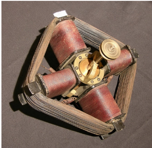
Fig. 1. Reconstruction of Galileo Ferraris' rotating magnetic field motor. Developed in the 1880s, Ferraris' design laid the foundation for the induction motor by demonstrating the generation of continuous rotary motion using two-phase alternating current (Istituto Elettrotecnico Nazionale Galileo Ferraris, Collezione antichi strumenti).
