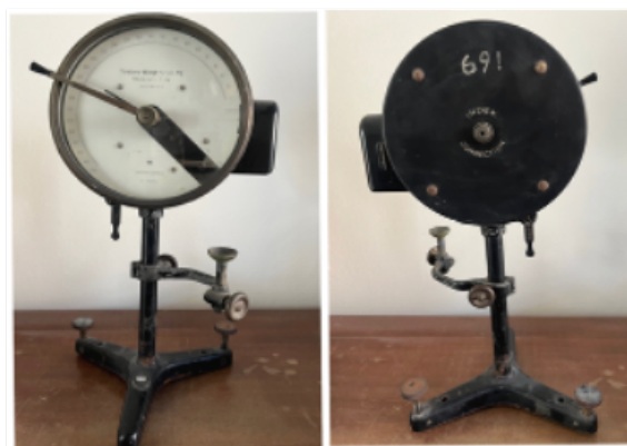
Fig. 2. Torsion Balance, Hartmann & Braun manufacturer, analysed by XRF and Raman.
