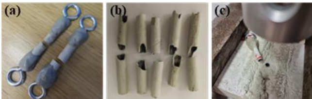
Figure 3. Capsules after (a) tensile, (b) flexural, and (c) bond tests performed in (Riordan et al. 2023).
