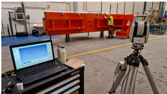
Fig. 13. Leica AT403 Measurement to validate the simulation on a real-world component.
