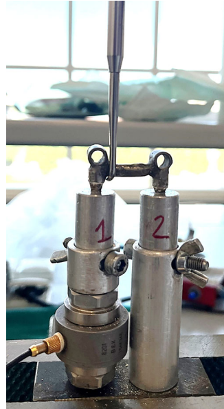
Figure 3. Bridge remover tip positioning during retrieval.
