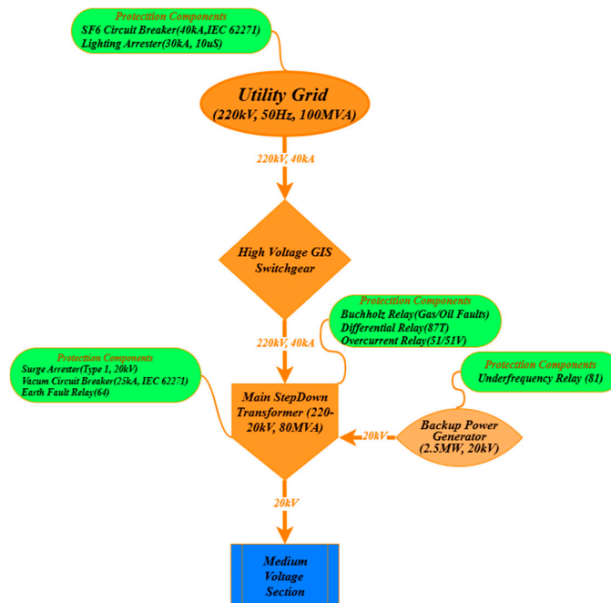
Figure 6. HV section of the power distribution network.
