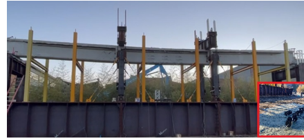
Fig. 4. Real framework testbed: 16 m-long beam from a decommissioned bridge. The bottom-right inset shows the cabling of electric sensors.
