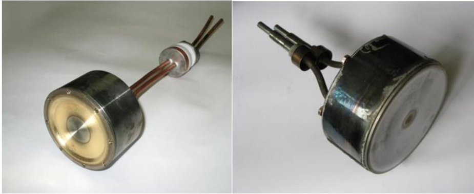
Figure 7. Photos of magnetron sputtering devices with a disk cooled cathode
