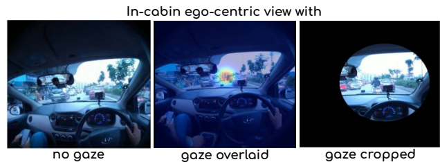
Figure 5. Variants of gaze input. The driver’s view video is processed in the following way to show the best way to represent gaze without affecting spatial features. The gaze cropped variant ( R = 350 ) produces the best quantitative results.
