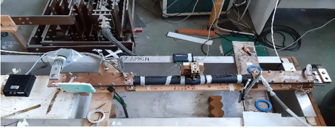
Fig. 2. The sample cable with the quench experiments equipment.
