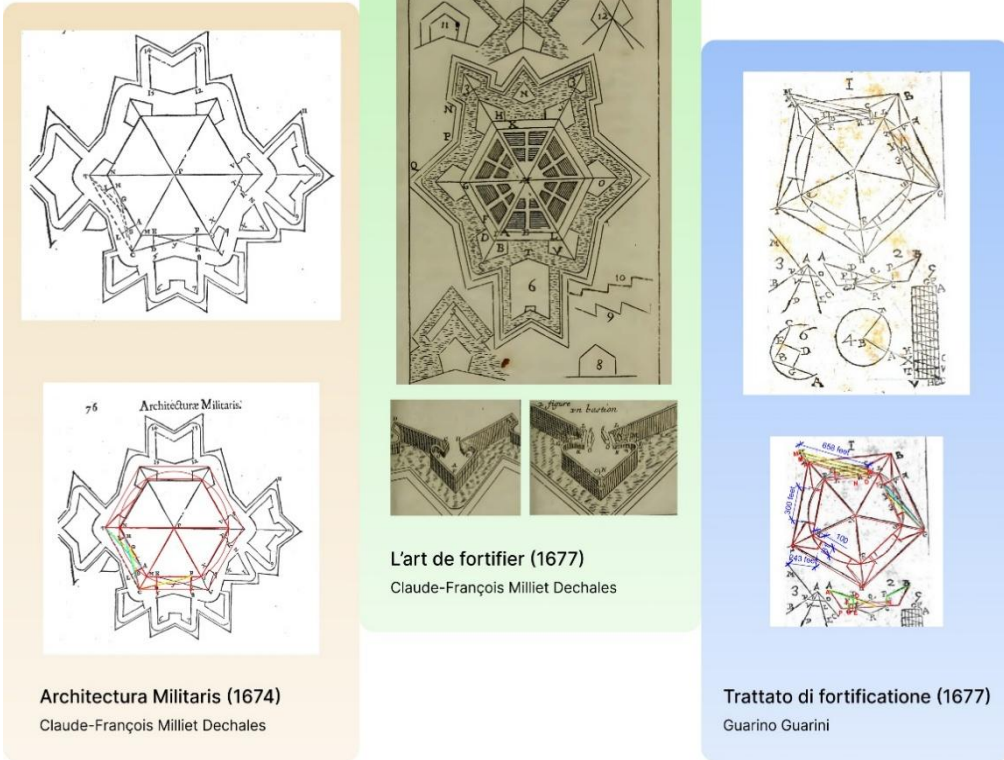
Fig. 3- Synoptic chart focusing on schematic drawings of fortified structures and the possible combinations of architectural elements (editing by Martina Rinascimento)
