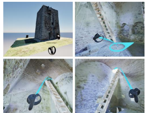
Fig. 8- VR experience test, accessible with 6 DoF navigation or a teleportation system (elaboration by E. Pupi, 2025)
