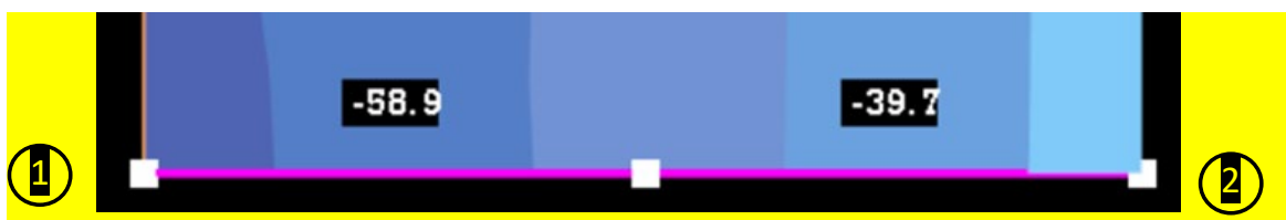
Fig. 3A. Section at the base of the wall depicted in the Dolmen, bounded by vertices 1 and 2, subjected to wind load acting along the X direction, with normal stresses in [daN/cm 2 ].
