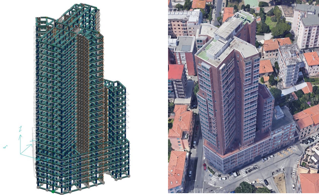
Fig. 9. FEM model made with CDM DOLMEN and view of the real structure.
