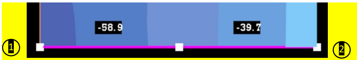
Fig. 3A. Section at the base of the wall depicted in the Dolmen, bounded by vertices 1 and 2, subjected to wind load acting along the X direction, with normal stresses in [daN/cm 2 ].
