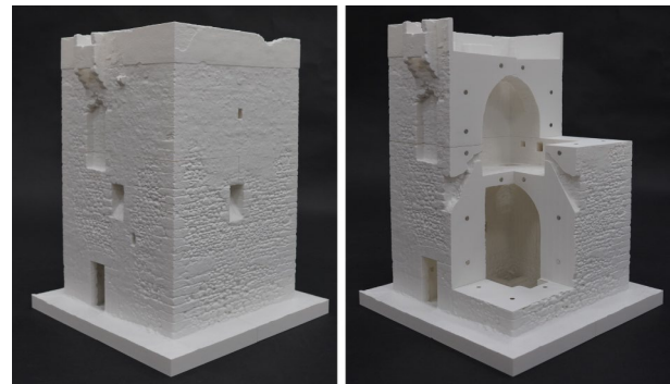
Figure 3. The 1:20-scale, 3D-printed, assembled modular replica (left) and a sectioned view (right). (Prototyping and photo: E. Pupi)
