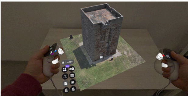
Figure 6. The MR environment using Gravity Sketch enables multi-scalar inspection and 3D annotation directly on the model. (Prototyping: E. Pupi)
