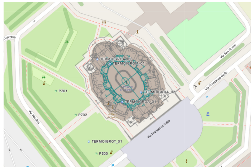
Figure 3. Location of the soil monitoring system (where TERMOIGRO “A”, “M” and “T” indicates the location of thermo-hygrometers for air, masonry and soil, and PZ the location of piezometers, the other terms in the figures define the names of the streets).
