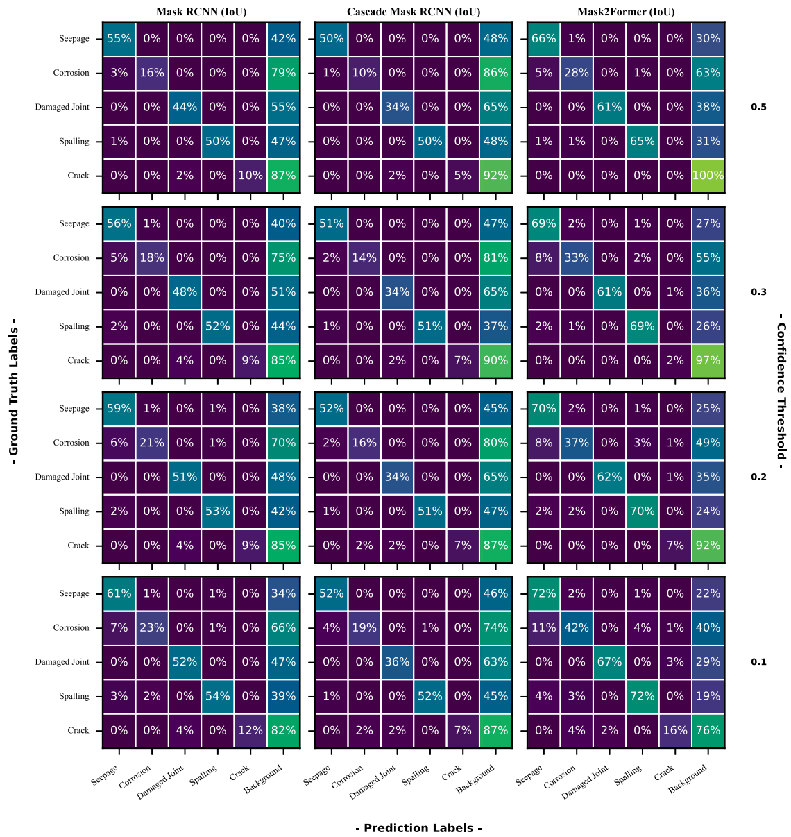
Fig. 12. Normalized confusion matrices of three instance segmentation algorithms based on IoU at different confidence thresholds.
