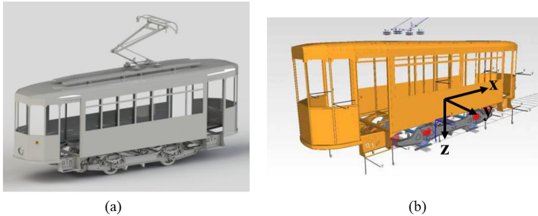
Figure 2: Reference tramway vehicle: (a) CAD drawing and (b) MB model with reference system axis.
